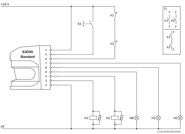
S3000 Standard in conjunction with relays/contactors
