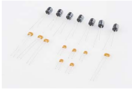
Electrolytic capacitors (top), ceramic capacitors (bottom).
