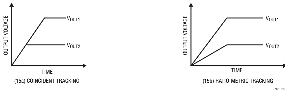
Figure 15. Two Different Methods of Output Voltage Tracking
