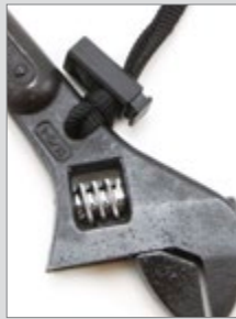
Attach tether through tether hole when available
