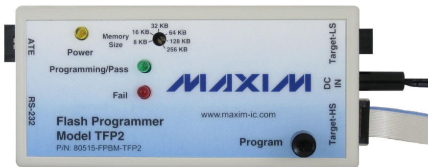
Figure 4-5: Standalone Configuration (shown with Target-HS cable)
