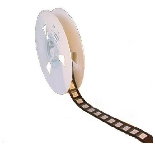
Figure 17: Reeled SARA-U2 modules
