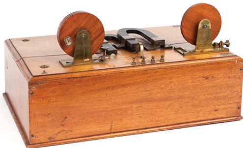
Figure 9. Magnetic detector as Marconi would have used. 3
