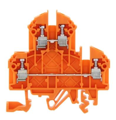
Double-level terminal, Screw connection, Mounting type:Mounting rail TS 35/7.5 and TS 32, Rated cross-section: 2.5 mm², Width: 5 mm, Colour: Orange
