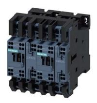
Reversing contactor assembly AC-3, 11 kW/400 V, 24 V DC 3-pole, Size S0 Spring-type terminal electrical and mechanical Interlock 2 NO integrated
