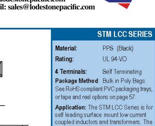
series will accommodate wound toroidal cores from .485 up to .605 in diameter and uses the toroid's winding leads to surface mount the toroid and case to
