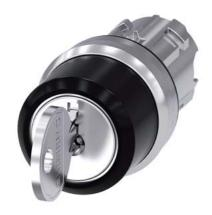
RONIS key-operated switch, 22 mm, round, metal, shiny, lock number SB30, with 2 keys, 3 switch positions I>O<II, momentary contact on the left, latching on the right, actuating angle 2x45°, 10:30h/12h/13:30h, key removal O, possible special locks: SB31, 421, 455, with laser labeling, lower case
