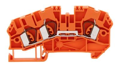
Feed-through terminal, Tension-spring connection, Mounting type: Mounting rail TS 35/7.5, Rated cross-section: 4 mm², Width: 6.1 mm, Colour: Orange
