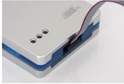
Figure 2-4. Atmel JTAGICE3 Cable Connection
