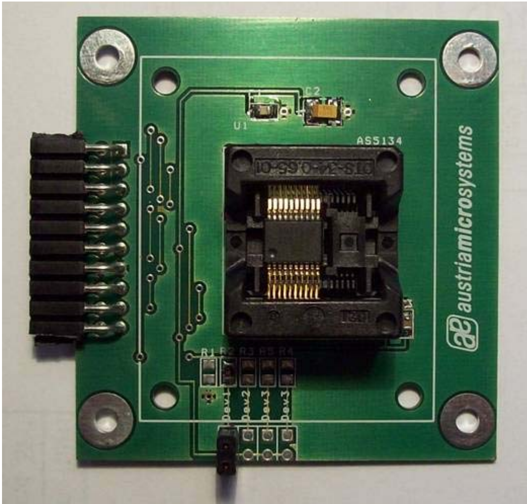
AS5134 360° Programmable High Speed BLDC Motor Commutation Magnetic Rotary Encoder Programming Board
