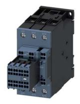
traction contactor, AC-3 51 A, 22 kW / 400 V 2 NO + 2 NC 110 V DC, 0.7-1.25\* US, with varistor, 3-pole, size S2, spring-loaded terminal
