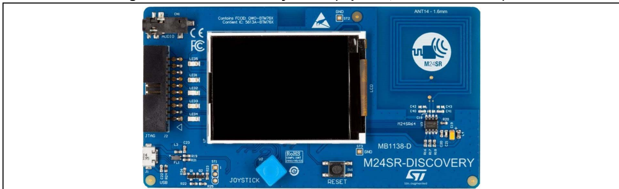
Figure 1. M24SR Discovery board (top side, Premium edition)
