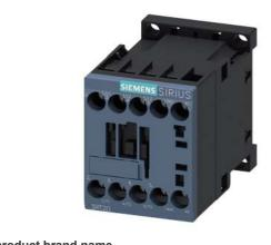
Power contactor, AC-3 7 A, 3 kW / 400 V 1 NO, 24 V AC, 50 / 60 Hz 3-pole, Size S00 screw terminal suspended mounting position
