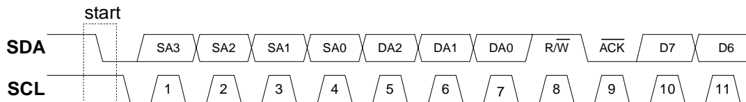
Figure 4-6. Addressing an I 2 C Peripheral
