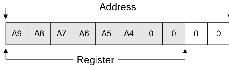
Figure 8-4. FIFO Start Address Format
