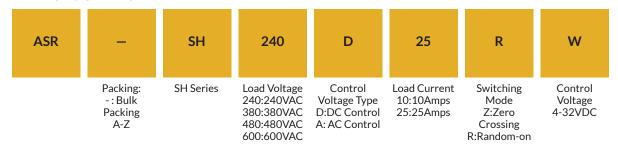
NOTE: Alternate control voltages: 18-36VAC, 4-15VDC, 15-32VDC are available as well as options for RC circuit and TVS. Consult with engineering to determine which combinations are available.
