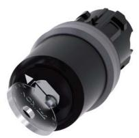
Key-operated switch IKON, 22 mm, round, plastic with metal front ring, special lock, with 2 keys, 2 switch positions O-I, latching, actuating angle 90°, 10:30h/13:30h, Key removal O
