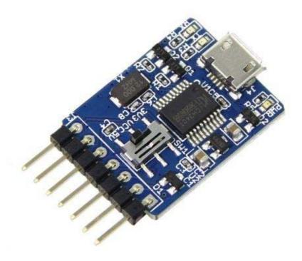
USB To Uart 5V/3V3 is a USB to serial adapter, Which is base on CH340, CH340 is a USB bus convert chip and it can realize USB convert to serial interface, USB convert to IrDA infrared or USB convert to printer interface. this module is compatible with 5V and 3v3.and it can used for upload code or communicating with MCUs.
