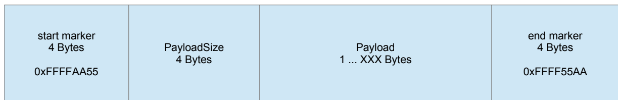
Figure 29: Command/Answer packet composition
