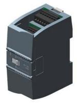
SIPLUS S7-1200 SM 1234 4Al/2AQ based on 6ES7234-4HE32-0XB0 with conformal coating, -20...+60 °C, analog I/O +/-10 V: 14-bit resolution or 0-20 mA: 13-bit resolution
