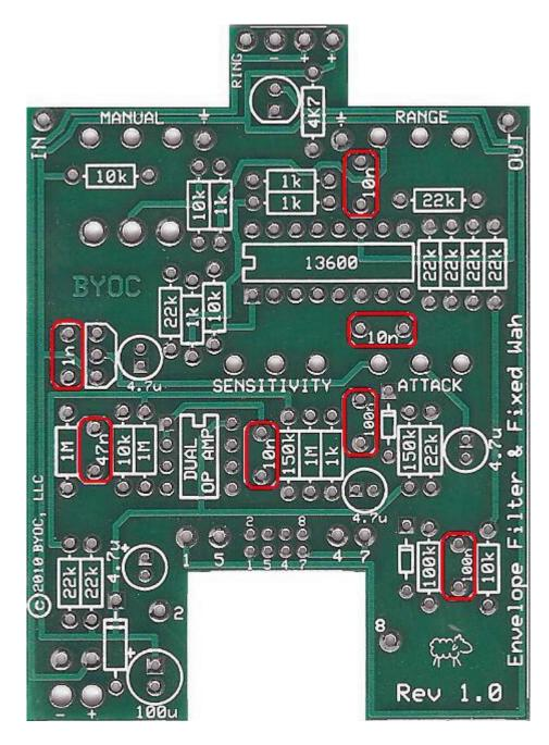
Step 5: Add the film capacitors. These are not polarized and can be inserted into the PCB either way.
