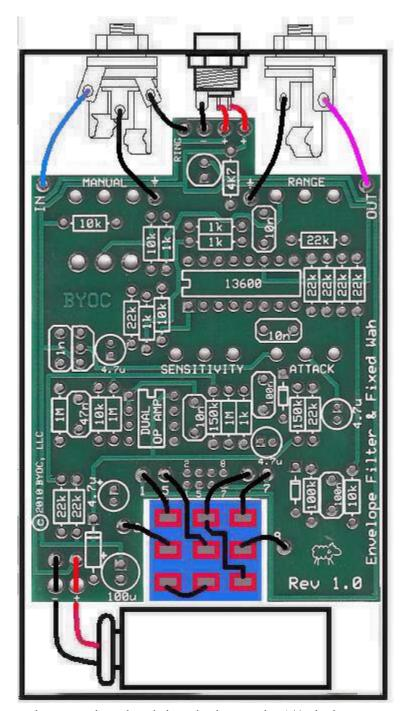
Step 3: Connect the pre stripped and tinned wires to the 1/4" jacks. Step 4:
