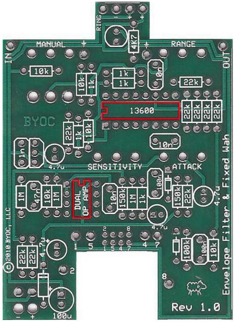
STEP 3: Add the 8 pin and 16 pin IC sockets. **ONLY SOLDER THE SOCKET! NOT THE ACTUAL IC!** These are sockets. The sockets get soldered to the PCB. The ICs get inserted into the sockets. The actual IC chips themselves, never get soldered. You will insert the ICs into the sockets after the entire pedal has been built.
