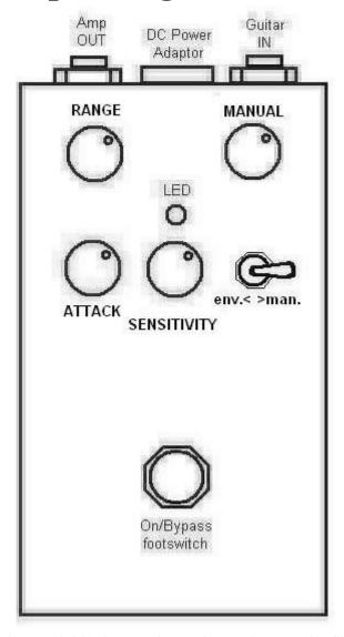
ATTACK: Controls how quickly the envelope trigger changes the filter
