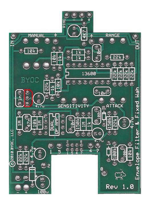
Step 4: Add the Transistor. Be sure to orient the transistor so that the flat side of the tansistor body matches up with the flat side on the PCB layout.
