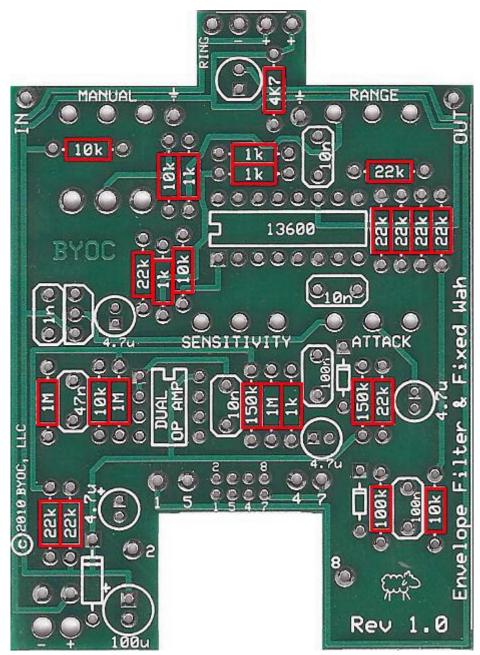
STEP 1: Add the resistors . Resistors are not polarized, so it does not matter which end goes in which solder pad.
