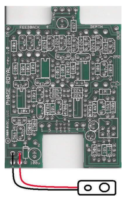
Step 7: Add the battery snap. Thread the solder ends of the battery snap into the strain relief holes from the bottom solderside of the PCB and out through the top. Insert the solder ends of the battery snap wires into the topside of their respective solder pads. Solder on the bottom side of the PCB. Remember the red wire goes in the "+" hole and the black wire goes in the "-" hole.
