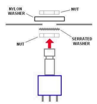
Step 2: Install the footswitch. Orient the footswitch so that the flat sides of the solder lugs are like the diagram below. NOTE: There are no actual number markings on the footswitch. There are two correct ways you can orient the footswitch. They are both 180
