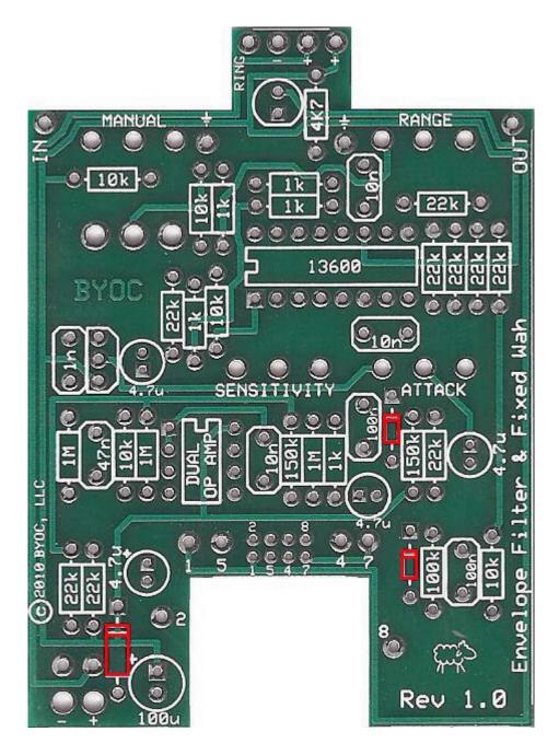
STEP 2: Add the diodes. Be sure to matched the end of the diode with the stripe to the layout on the PCB. The stripped end should go in the square solder pad. The black plastic 1N4001 diode goes in the larger diode space. The orange glass 1N4148 diodes go in the smaller diode spaces.
