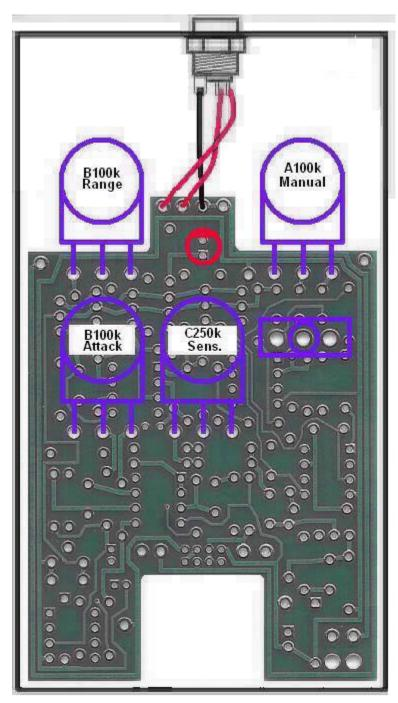
Step 3: Flip the PCB over so that the bottom or solder side is up. Insert the 2 x B100k(range & attack),C250k(sensitivity), A100K(manual) potentiometers, the SPDT toggle switch, and the LED into the bottom side of the PCB. DO NOT SOLDER ANYTHING YET!!! The LED will have one lead that is longer than the other. The longer lead goes in the hole with the square solder pad.
