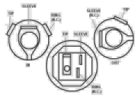
Step 1: Install the 1/4" jacks to the enclosure. Be sure to turn the OUT jack a 1/4 turn counter clockwise so that solder terminal for the tip does not short out against the enclosure.
