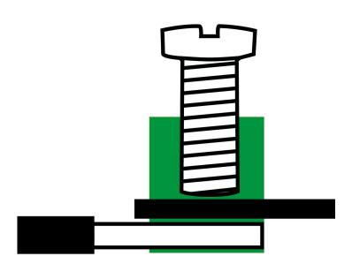
Feed-through terminal, Screw connection, Mounting type: Mounting rail TS 35/7.5, Rated cross-section: 10 mm², Width: 8 mm, Colour: Green
