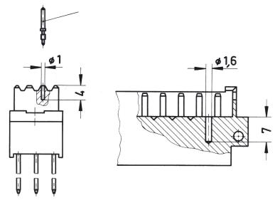
To avoid cross-plugging of adjacent connectors a coding system is required.
