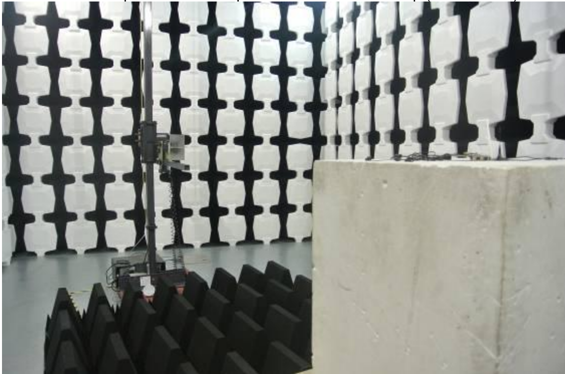
Description: Radiated Spurious Measurement Setup (Above 1GHz)
