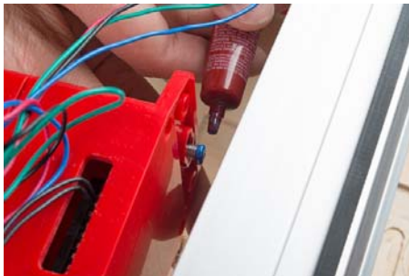
Applying threadlocker – Here, a bit too much is used. It only needs to be filling in the treads. Excess may run.
