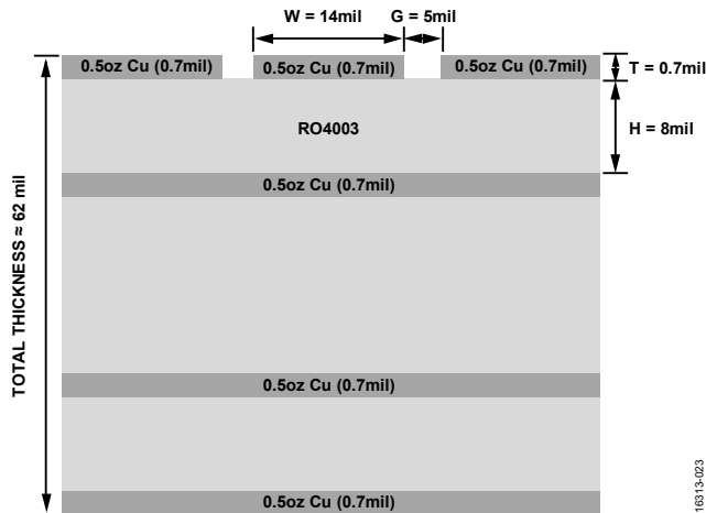
Figure 23. Evaluation Board (Cross Sectional View)
