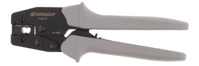
Crimping tool for crimping wire-end ferrules with and without plastic collars. Cross-section range: 50 mm<sup>2</sup>. Easy to use, Auto-lock for proper and complete crimping, Wire can be fed in from the side, Self-opening with built-in spring.
