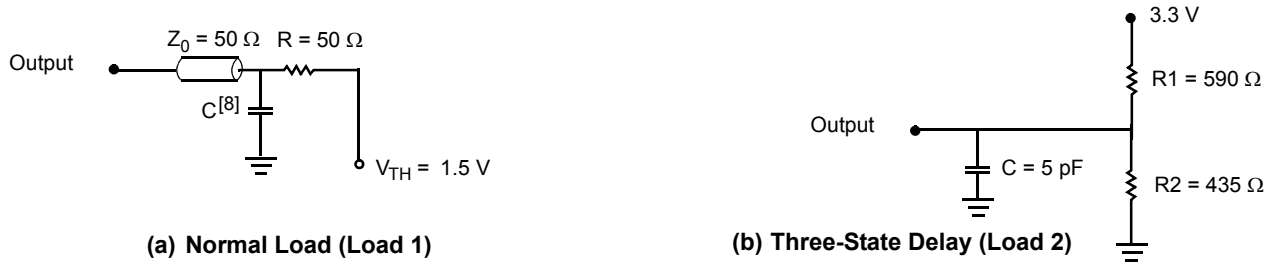
Figure 3. AC Test Load and Waveforms
