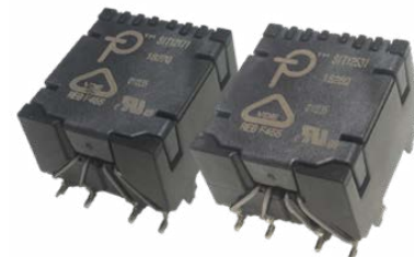
Figure 2. SIT1217I and SIT1253I Transformers.
