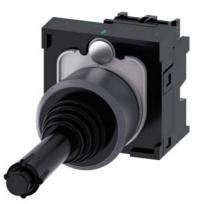
Coordinate switch, 22 mm, round, plastic with metal front ring, black, 2 switch positions, vertical latching, with mechanical interlocking, in O position, with holder, 1 NO, 1 NO, screw terminal,
