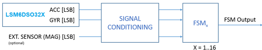
Figure 2. State machine in the LSM6DSO32X
