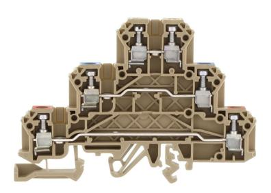
Three-level initiator terminal | Multi-wire terminal, Screw connection, Mounting type:Mounting rail TS 35/7.5 and TS 32, Rated cross-section: 2.5 mm², Width: 5 mm, Colour: Beige
