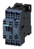
Traction contactor, AC-3 38 A, 18.5 kW / 400 V 1 NO + 1 NC with solid-state operating mechanism 24 V DC, 0.7-1.25\* Us with integrated varistor 3-pole Size S0, Spring-type terminals
