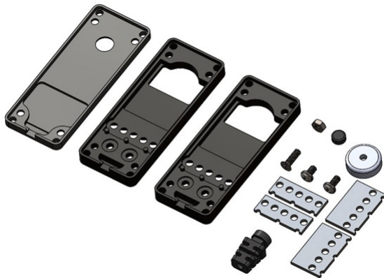
Figure 68: The hardware components of the clamp enclosure kit are shown. For simplicity the actual wiring, and some of the repeated bolts etc are not shown.
