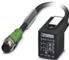
Sensor/Actuator cable, 3-position, PUR halogen-free, Black-gray RAL 7021, Plug straight M12, A-coded, on BI valve plug (11 mm), with 1 LED, connected with Z diode, Cable length: 1.5 m
