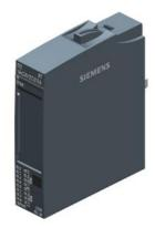
SIMATIC ET 200SP, Digital output module, DQ 16x 24V DC/0.5A STANDARD, Source output (PNP,P-switching) Packing unit: 10 pieces, fits to BU-type A0, Colour Code CC00, substitute value output, module diagnostics for: short-circuit to L+ and ground, wire break, supply voltage
