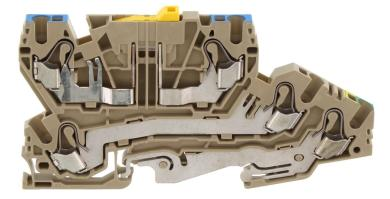
Three-wire installation terminal, Push-in connection, Mounting type: Mounting rail TS 35/7.5, Rated cross-section: 4 mm<sup>2</sup>, Width: 5.1 mm, Colour: Beige
