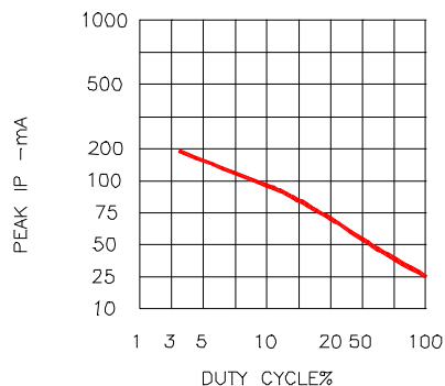
DUTY CYCLE% Fig.6 MAX PEAK CURRENT VS. DUTY CYCLE % (REFRESH RATE f=1KHz)
