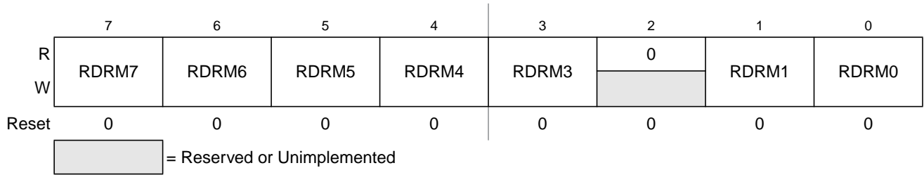
Figure 3-13. Port M Reduced Drive Register (RDRM)
