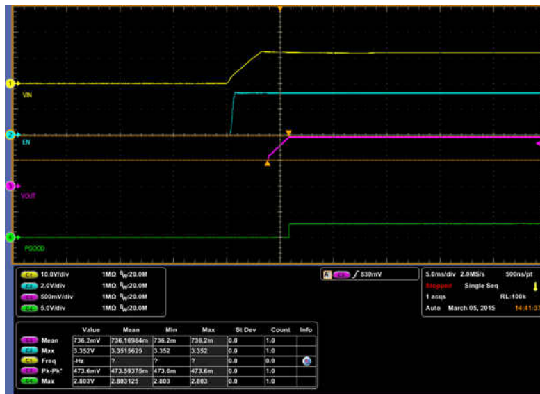
Figure 8-7. Start up from Control, 0.95-V Output at 12 V_{IN} , 20-A Output
