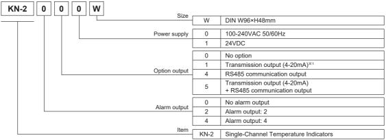
%1: For transmission output(4-20mA), select one between transmission output+alarm output 2 or transmission output+alarm output 4.
