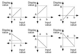
Display scale function is able to change display value for max./min. measured input by setting high limit scale [H-5L] and low limit scale [L-5L] in program mode. XE.g.) Set high/low scale value (input range is 0 to 10V)
