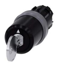
Key-operated switch BKS, 22 mm, round, plastic with metal front ring, Lock No. E2 (VW), without key, 3 switch positions I-O-II, latching, actuating angle 2x45°, 10:30h/12h/13:30h, Key removal I+O+II, with laser labeling, inscription or symbol Customer-specific selection with SIRIUS ACT configurator (CIN)
