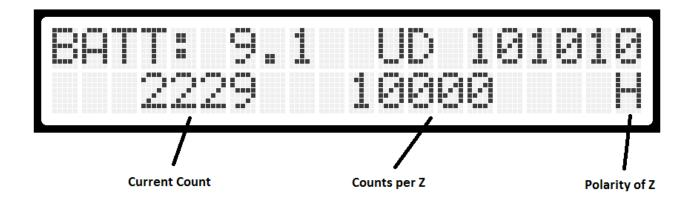
The polarity of Z show the first change in state for the Z signal. If the Z is normally low, it will pulse high and show an "H" there.
