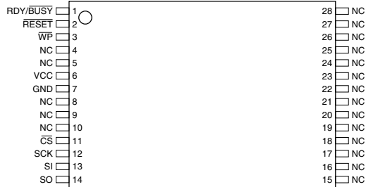
Figure 2-1. TSOP Top View, Type 1
