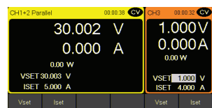
Channel 1+2 parallel view
