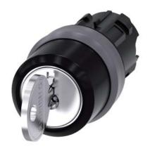
RONIS key-operated switch, 22 mm, round, plastic with metal front ring, lock number SB30, with 2 keys, 3 switch positions I>O<II, momentary contact on the left, latching on the right, actuating angle  $2x45^{\circ}$ , 10:30h/12h/13:30h, Key removal II, possible special locks: SB31, 421, 455, Z=50-unit packaging
