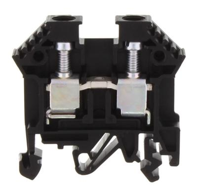
Feed-through terminal, Screw connection, Mounting type:Mounting rail TS 35/7.5 and TS 32, Rated cross-section: 10 mm², Width: 8 mm, Colour: Black
